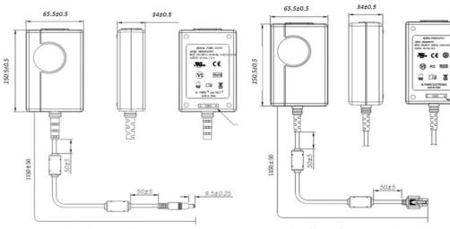
$$15\rm{V}$$  through 24V Models  $2.5\rm{mm}\times5.5\rm{mm}\times9.5\rm{mm}$  Barrel Connector, center positive
