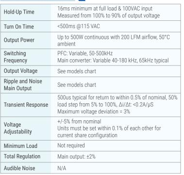
Note: Unless is stated otherwise, all specification are based on 25°C ambient.
