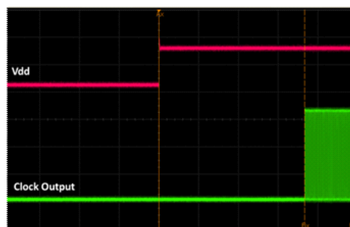
Figure 17. Startup Waveform vs. Vdd
