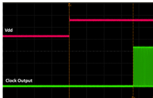
Figure 16. Startup Waveform vs. Vdd
