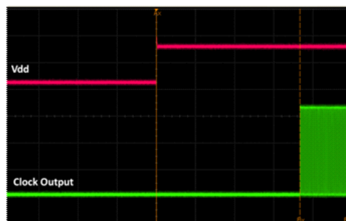
Figure 17. Startup Waveform vs. Vdd
