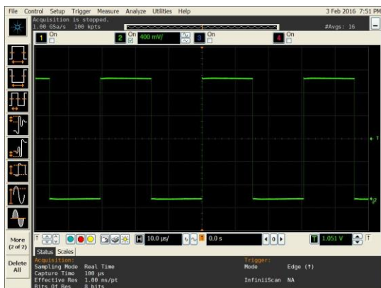
Figure 3. LVC MOS Output Swing ( V_{DD} = 1.8\text{ V} )
