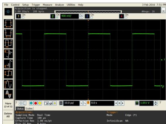
Figure 3. LVCMOS Output Swing ( V_{DD} = 1.8\text{ V} )
