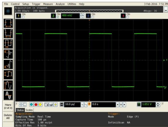
Figure 3. LVC MOS Output Swing ( V_{DD} = 1.8\text{ V} )
