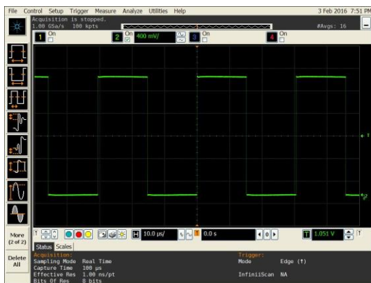
Figure 7. LVCMOS Output Sing
