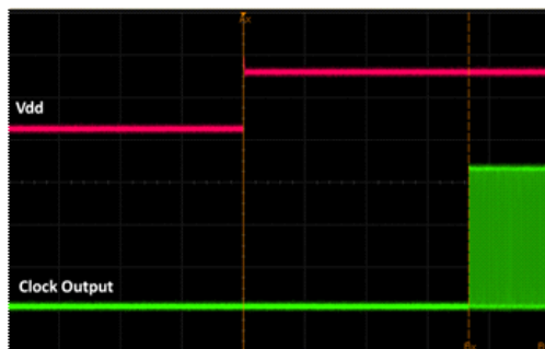
Figure 17. Startup Waveform vs. Vdd
