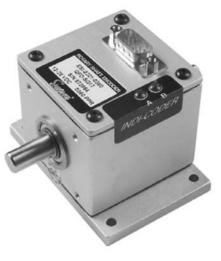
To aid in troubleshooting, LEDs are located directly on the body to instantly verify correct output operation. Quadrature output is standard and can be externally scaled to provide any engineering unit (RPM, angular position, feet/min., etc.). Gold-plated connectors ensure maximum signal transfer. Very low power consumption; typical current draw, 35mA @ 15DCV.
