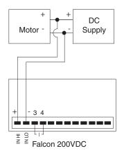
dard feature on the Falcon. By shorting connections #3 and #4, the operator can hold the display to take a reading, and then remove the short to reactivate the indication mode.
