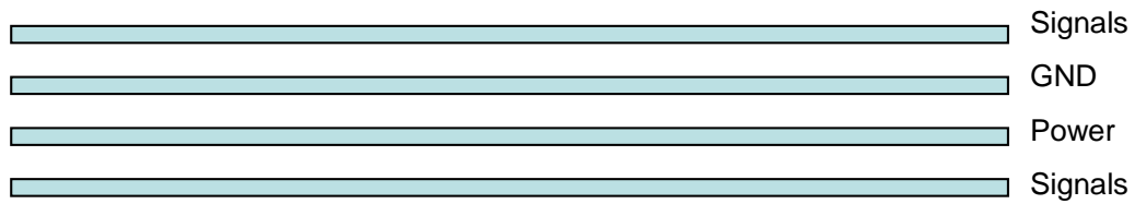
Figure 17: Typical 4-layer PCB construction
