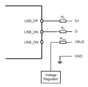
Figure 23: USB Connections for Bus-Powered Mode
