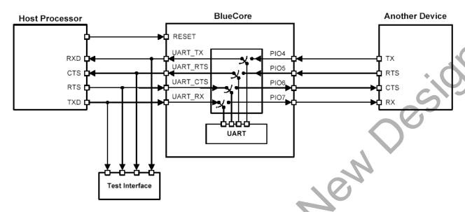
Figure 20: UART Bypass Architecture
