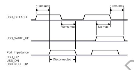
Figure 24: USB\_Detach and USB\_Wake\_Up Signals
