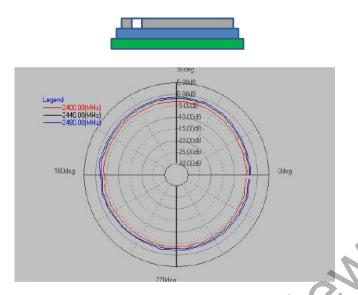
Figure 5: Antenna radiation pattern in a USB dongle layout
