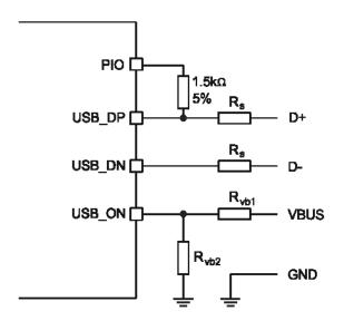
Figure 21: USB Connections for Self-Powered Mode
