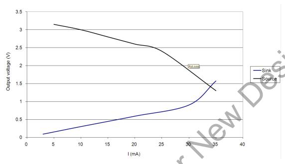
Figure 2: WT11u PIO Current Drive Capability
