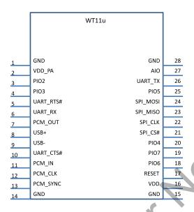
Figure 1: WT11u connection diagram
