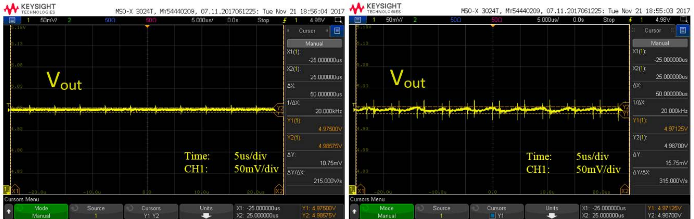
Figure 7.1. Si3404 Isolated Flyback EVB Output Voltage Ripple at No Load (Left) and Heavy Load (Right) Conditions
