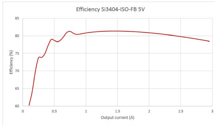
Figure 3.1. Si3404 Isolated Flyback EVB Overall Efficiency: 50 V Input, 5 V Output, Class 3
