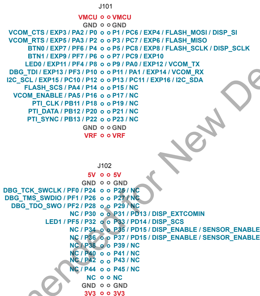
Figure 3.2. Radio Board Pin Mapping on Breakout Pads
