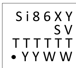
Figure 16.1. DFN-8 Top Marking
