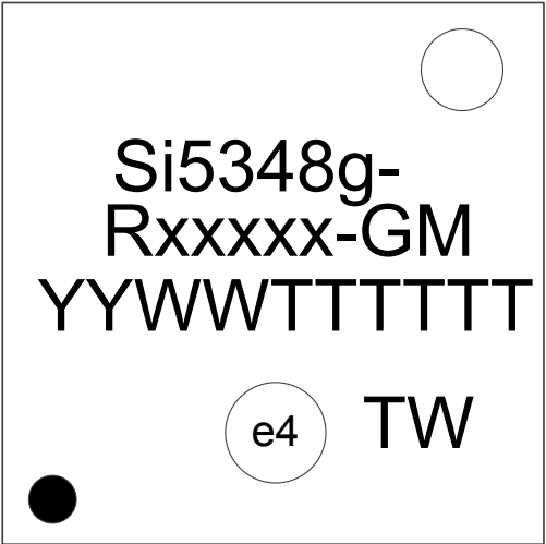
Figure 13.1. Si5348 Top Marking
