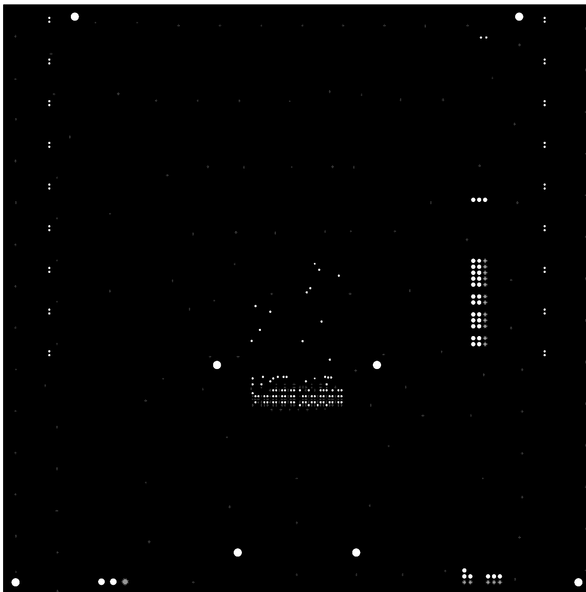
Figure 47. Layer 2—GND1 Plane (Optional Full-Duplex Motherboard)
