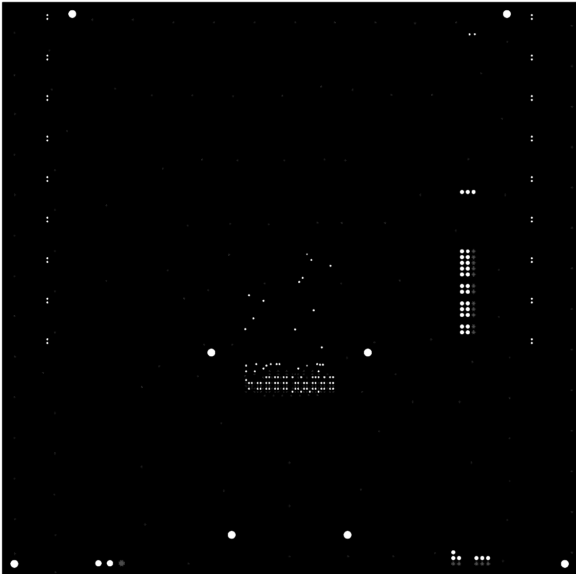
Figure 50. Layer 5—GND2 Plane (Optional Full-Duplex Motherboard)
