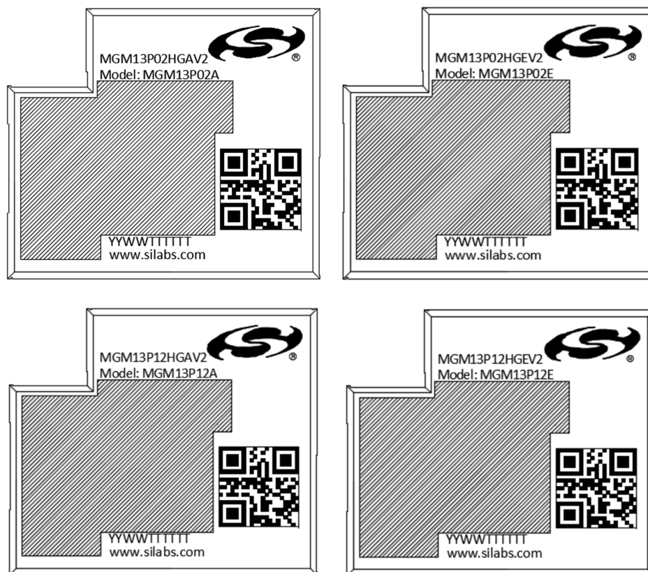
Figure 9.5. MGM13P Package Marking
