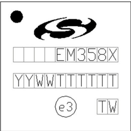
Figure 6.7. Part Marking for EM358x
