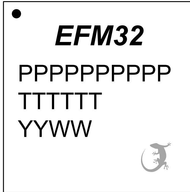
Figure 12.3. QFN64 Package Marking
