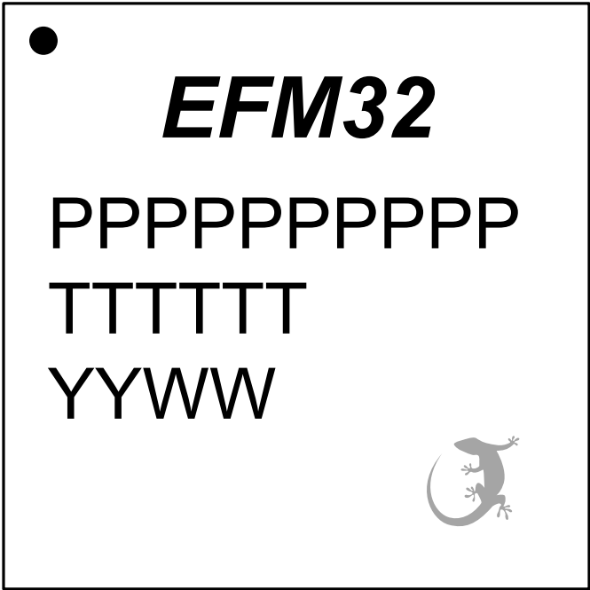
Figure 11.3. TQFP64 Package Marking
