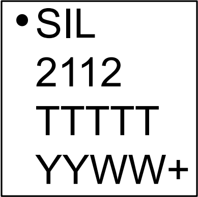
Figure 5.3. QFN24 Package Marking
