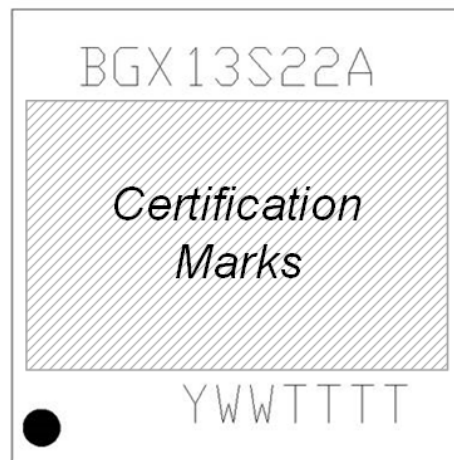
Figure 7.4. BGX13S Package Marking
