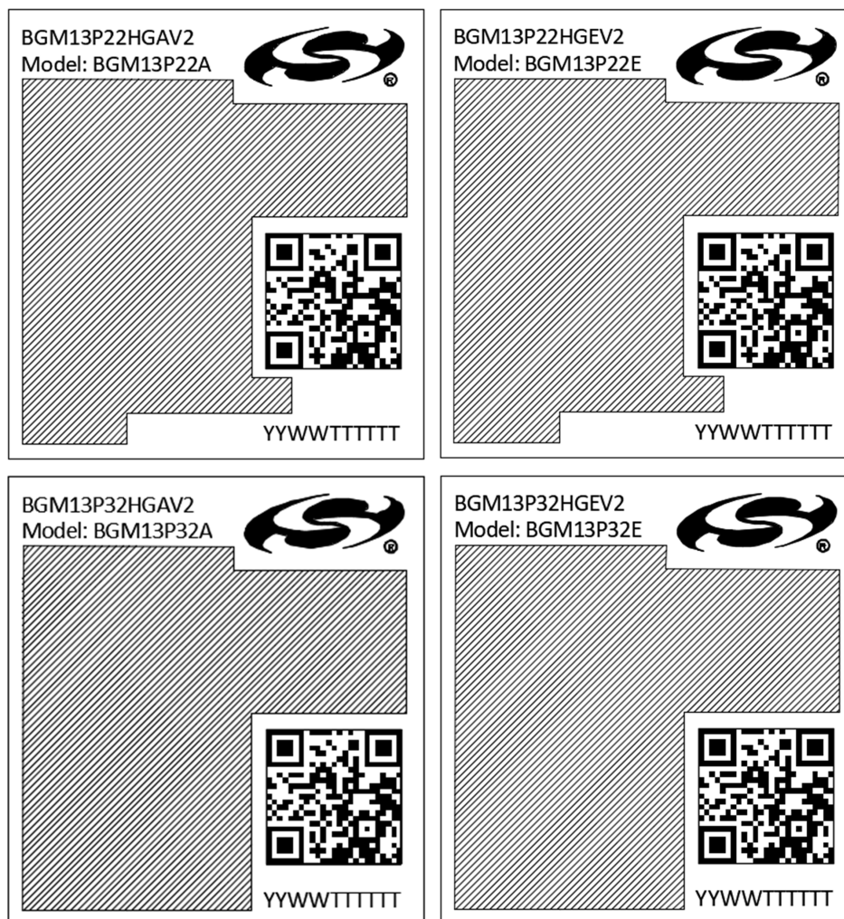
Figure 9.5. BGM13P Package Marking
