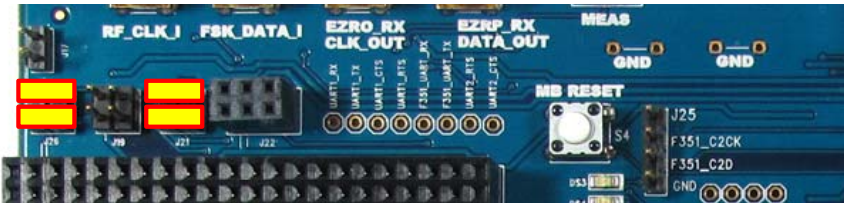
Figure 17. Radio Power Headers Diagram (EBID Powered by 5 V)
