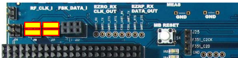
Figure 16. Radio Power Headers Diagram (EBID Powered by 3.3 V)
