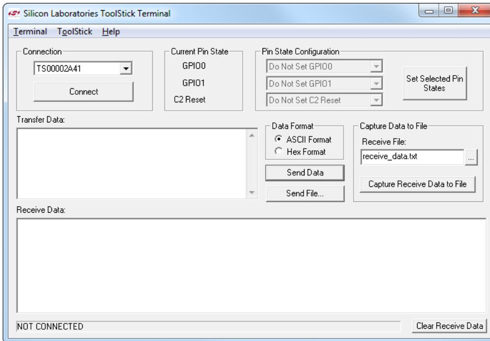
4. In the top, left-hand corner of the Terminal application, available devices are shown in the drop-down Connection menu. Click **Connect** to connect to the device.
