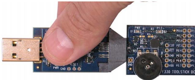
Figure 2. Improper Method of Holding the ToolStick
