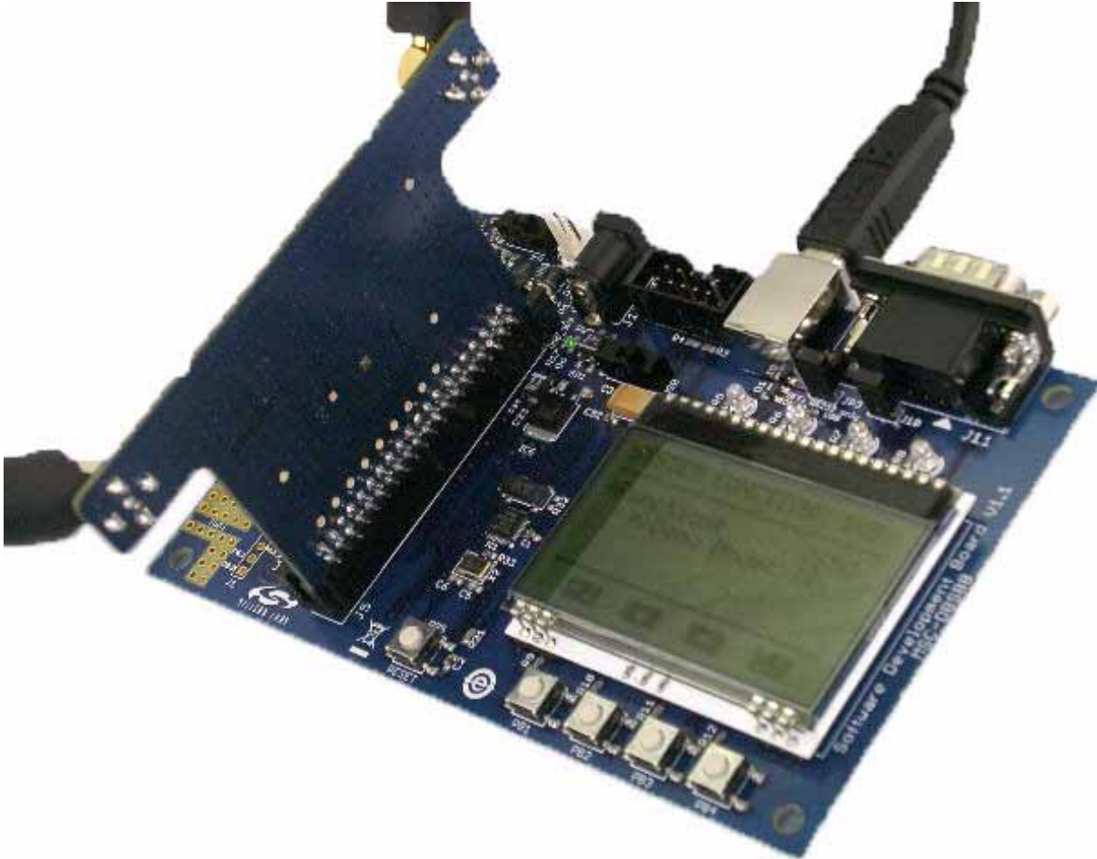
Figure 7. Software Development Board (MSC-DBSB8) with a Standard Silicon Labs Testcard Installed
