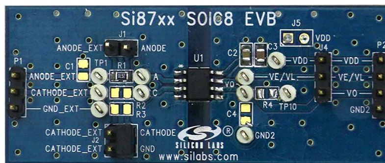
Figure 2. Si871x SOIC8 Evaluation Board Overview
