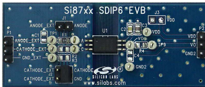
Figure 3. Si871x SDIP6 Evaluation Board Overview
