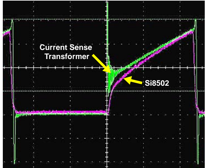
Figure 8. Leading-Edge Noise Suppression Waveforms (200 kHz, 9.3 A Load)
