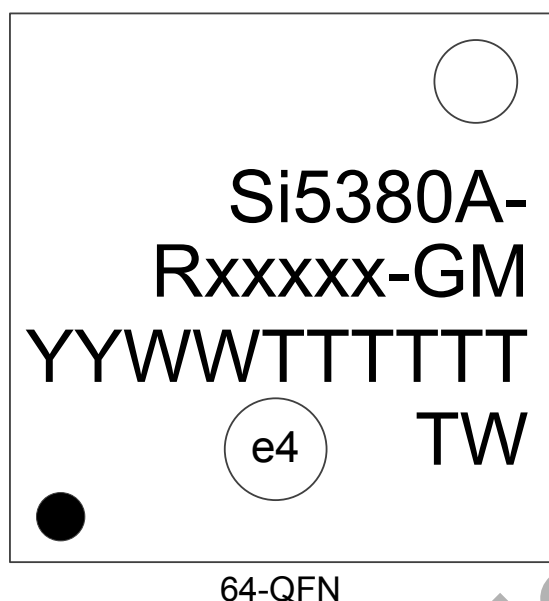
Figure 12.1. Si5380 Top Marking
