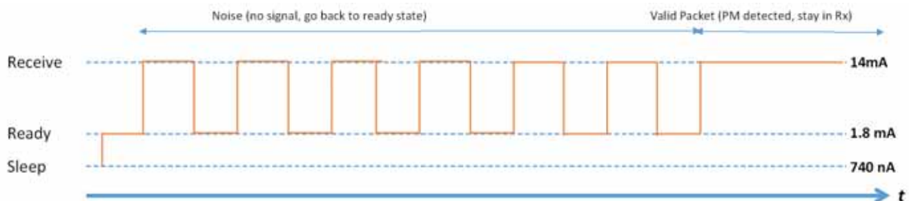
Figure 15. Preamble Sense Mode
