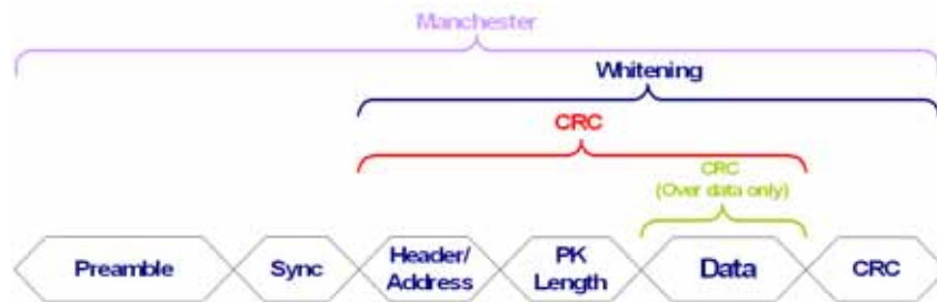
Figure 14. Operation of Data Whitening, Manchester Encoding, and CRC
