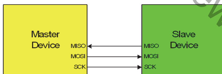
Figure 25.3. 3-Wire Single Master and 3-Wire Single Slave Mode Connection Diagram
