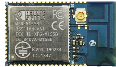
LGA Module (AA1) 27 mm x 16 mm
