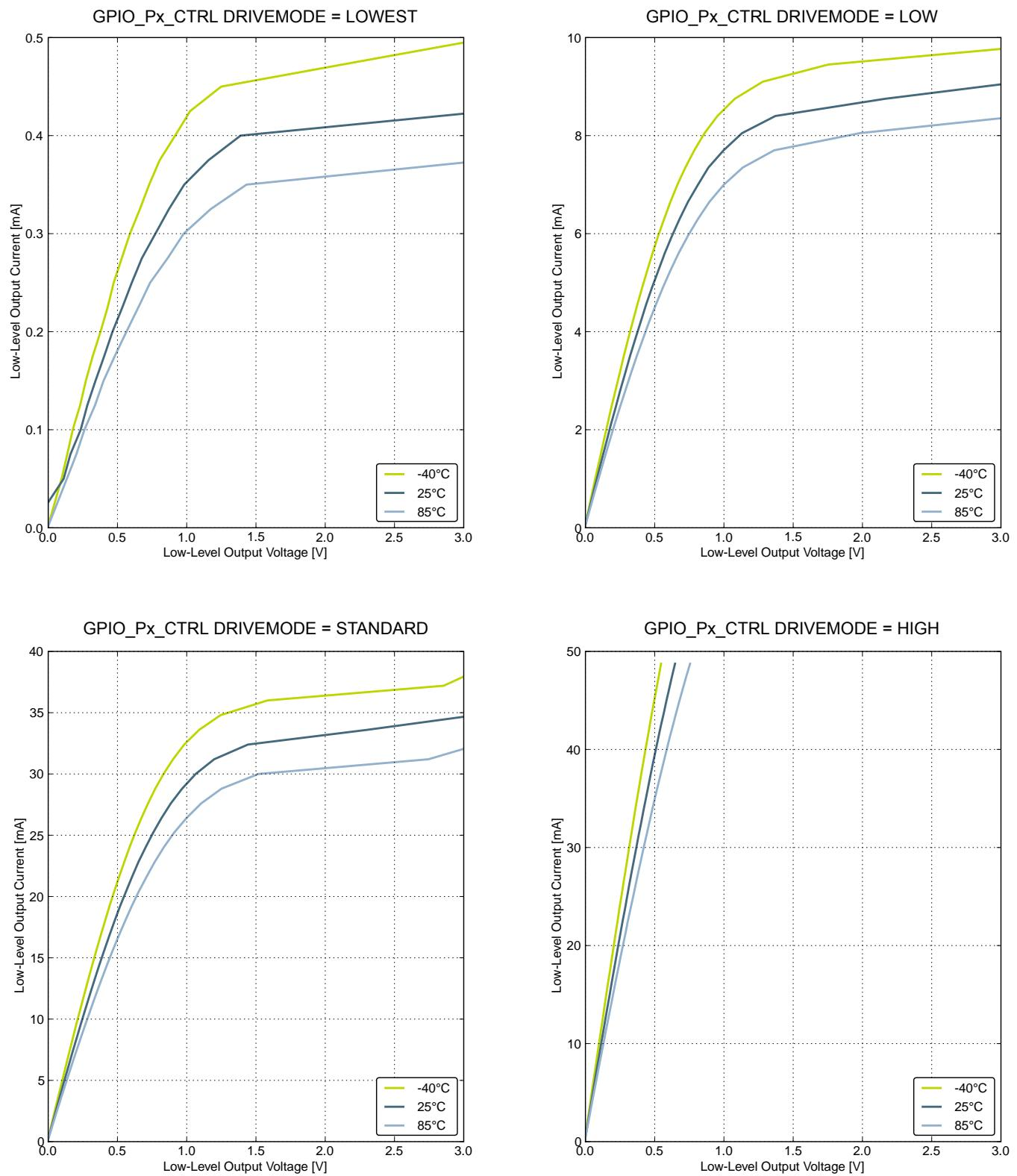
**Figure 4.16. Typical Low-Level Output Current, 3V Supply Voltage**
