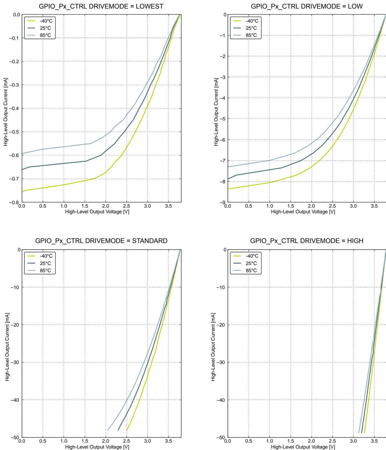
Figure 4.19. Typical High-Level Output Current, 3.8V Supply Voltage
