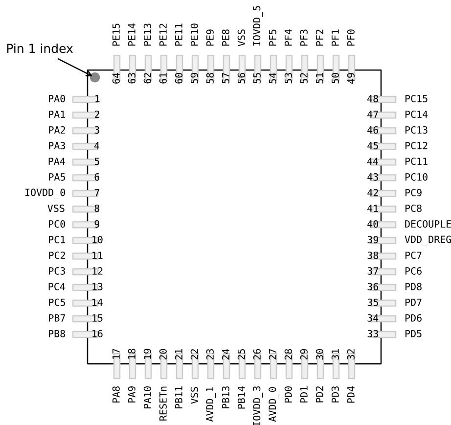
Figure 5.4. EFM32G232 Pinout (top view, not to scale)
