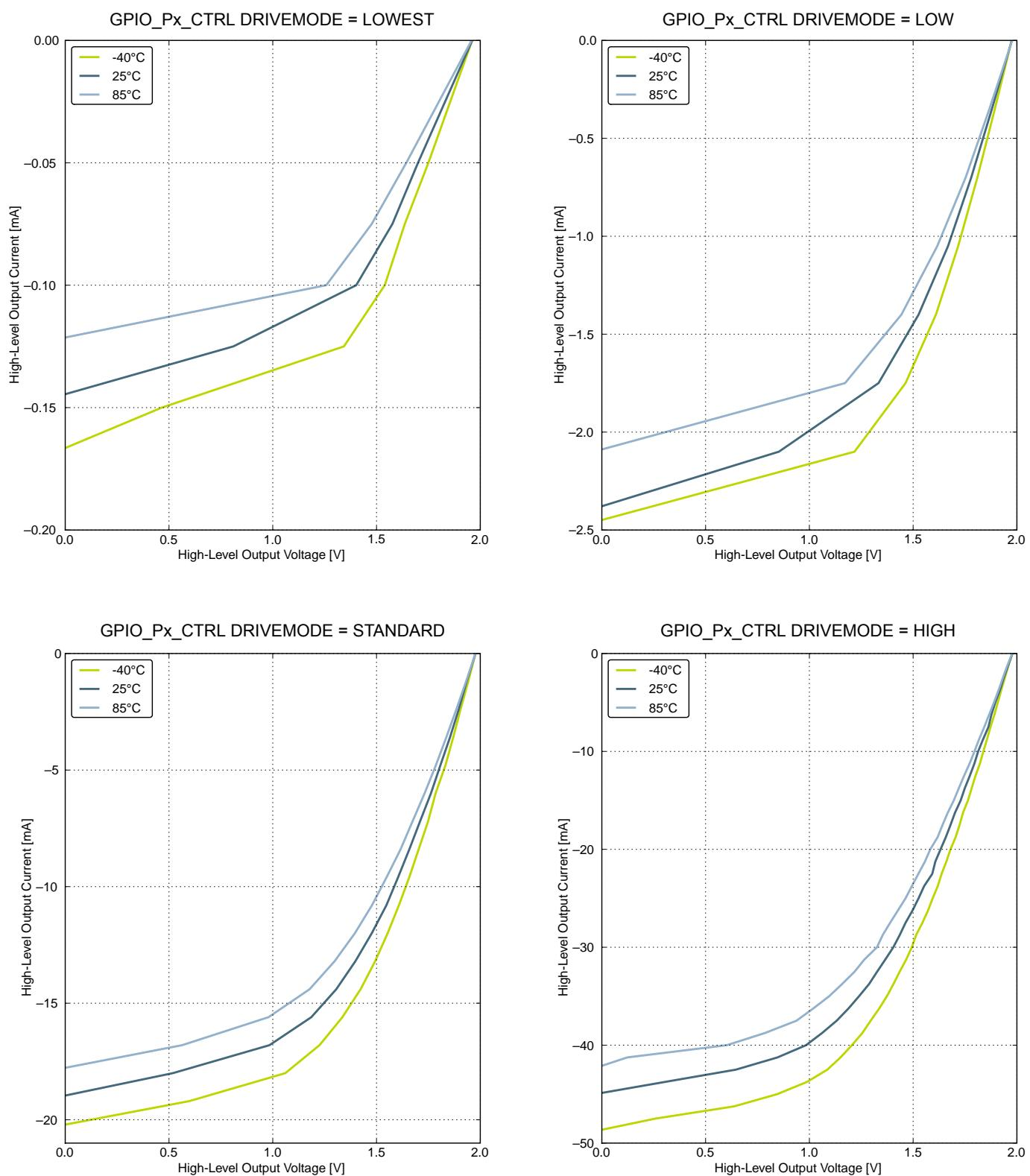
Figure 4.15. Typical High-Level Output Current, 2V Supply Voltage
