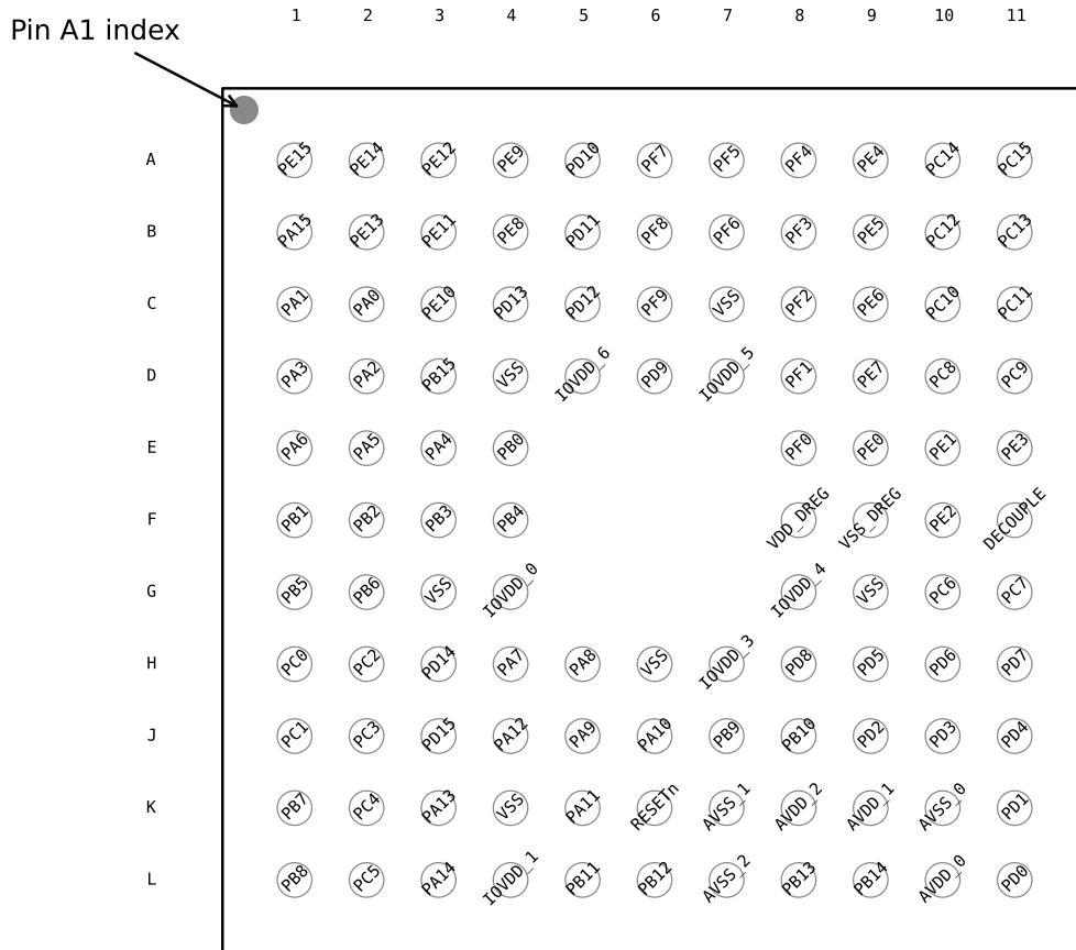
**Figure 5.6. EFM32G280 Pinout (top view, not to scale)**
