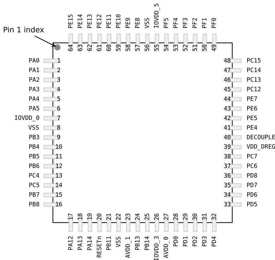
Figure 5.8. EFM32G842 Pinout (top view, not to scale)
