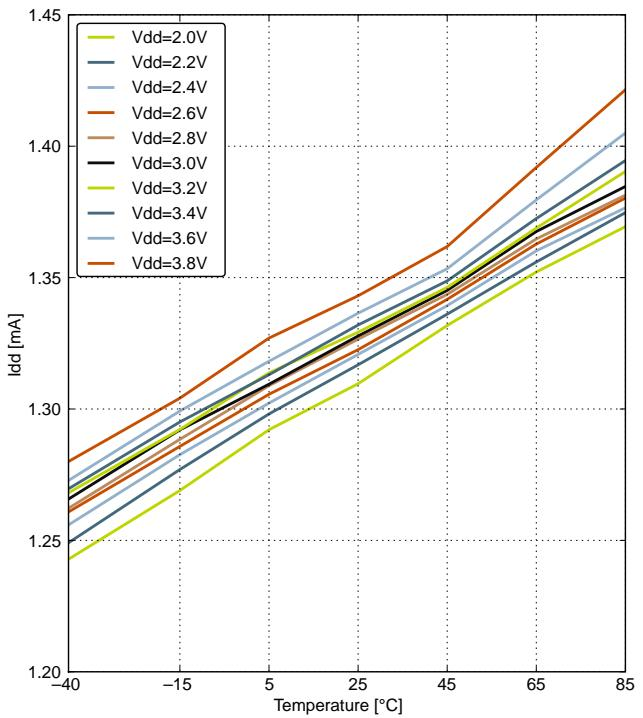
**Figure 4.5. EM0 Current consumption while executing prime number calculation code from flash with HFRCO running at 7 MHz**
