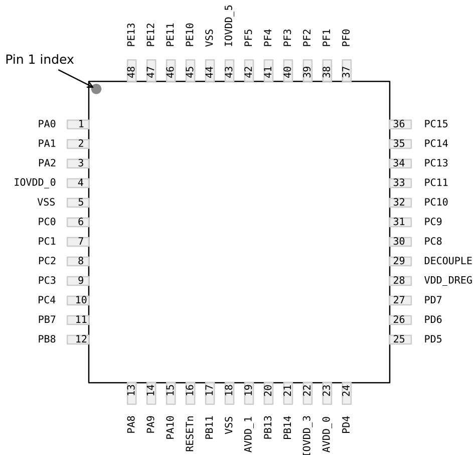
**Figure 5.2. EFM32G222 Pinout (top view, not to scale)**
