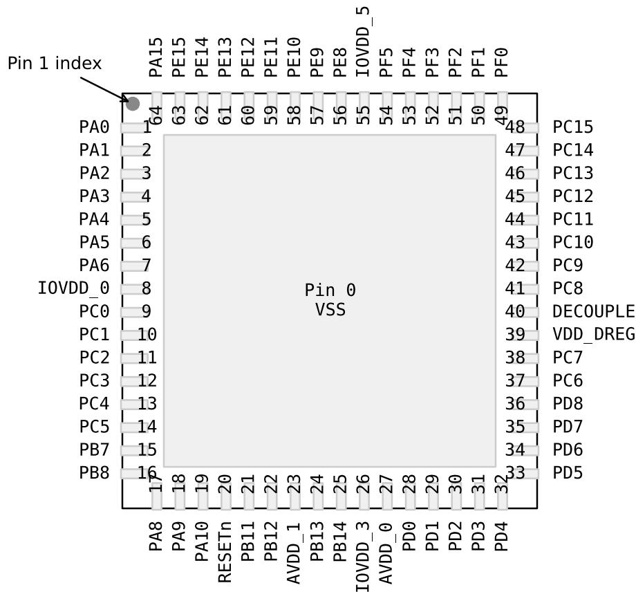
Figure 5.3. EFM32G230 Pinout (top view, not to scale)
