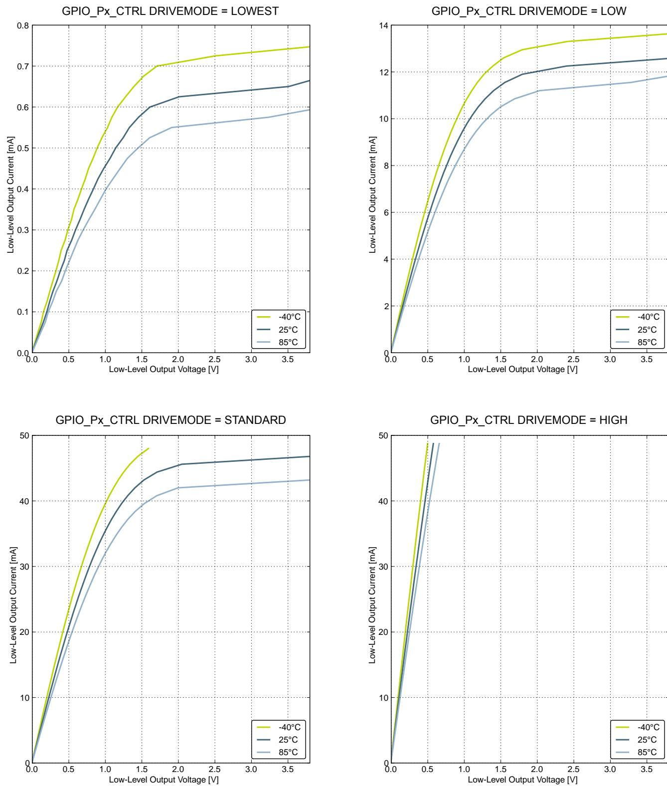
Figure 4.18. Typical Low-Level Output Current, 3.8V Supply Voltage
