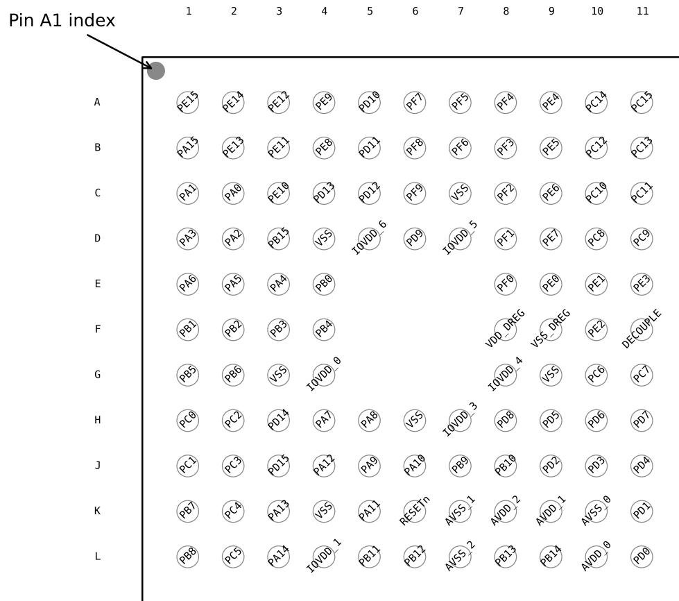
**Figure 5.10. EFM32G890 Pinout (top view, not to scale)**
