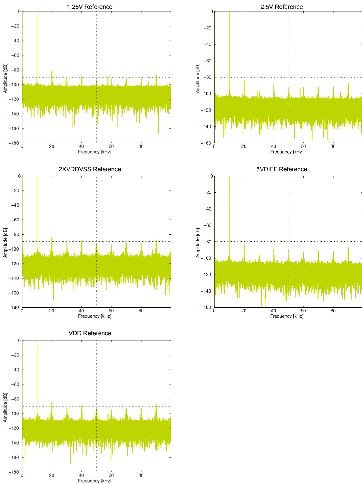
Figure 4.29. ADC Frequency Spectrum, VDD = 3V, Temp = 25°C
