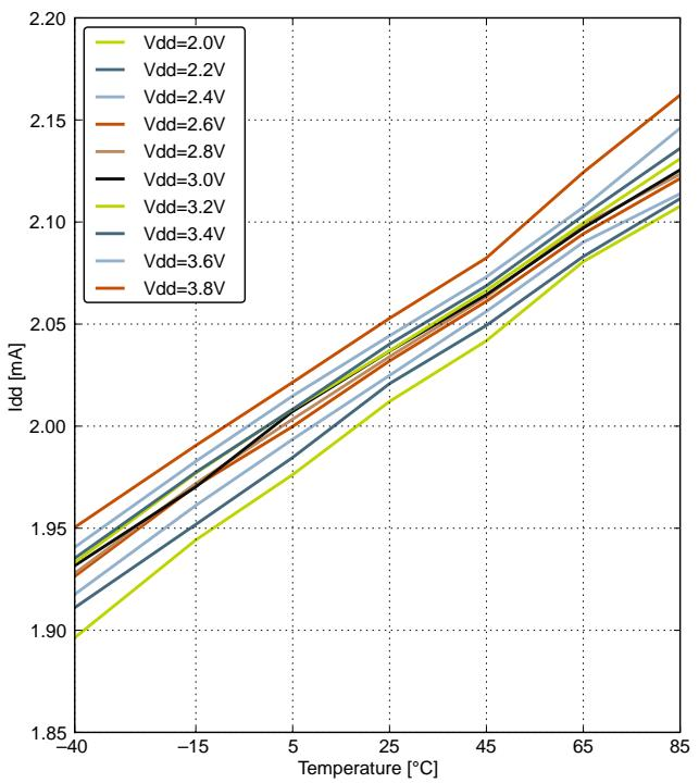
**Figure 4.4. EM0 Current consumption while executing prime number calculation code from flash with HFRCO running at 11 MHz**
