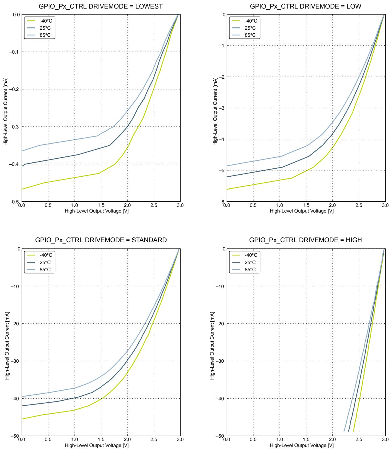
**Figure 4.17. Typical High-Level Output Current, 3V Supply Voltage**
