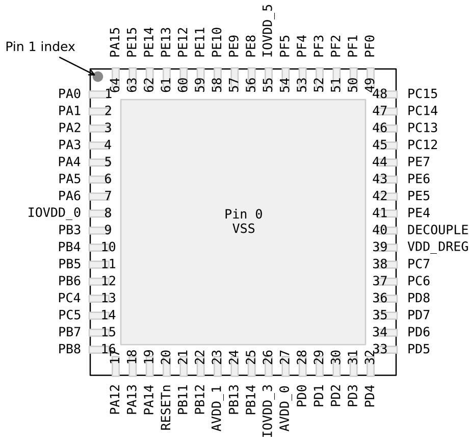
Figure 5.7. EFM32G840 Pinout (top view, not to scale)
