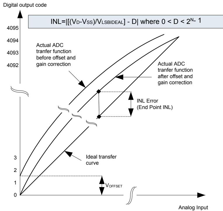
**Figure 4.27. Integral Non-Linearity (INL)**
