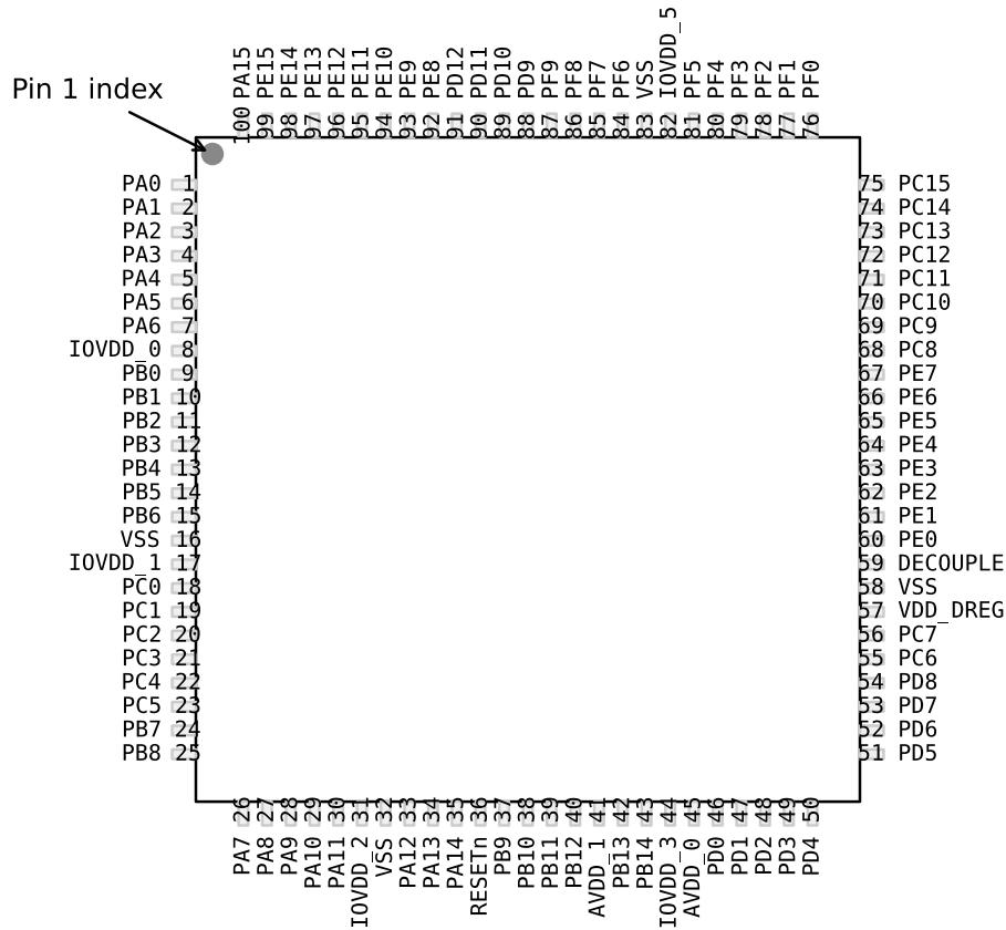
Figure 5.9. EFM32G880 Pinout (top view, not to scale)
