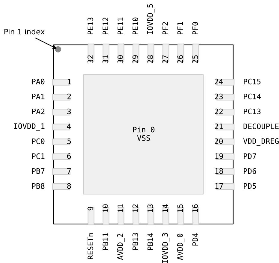
Figure 5.1. EFM32G200 & EFM32G210 Pinout (top view, not to scale)
