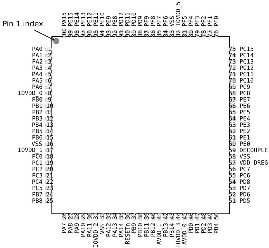
Figure 5.5. EFM32G280 Pinout (top view, not to scale)
