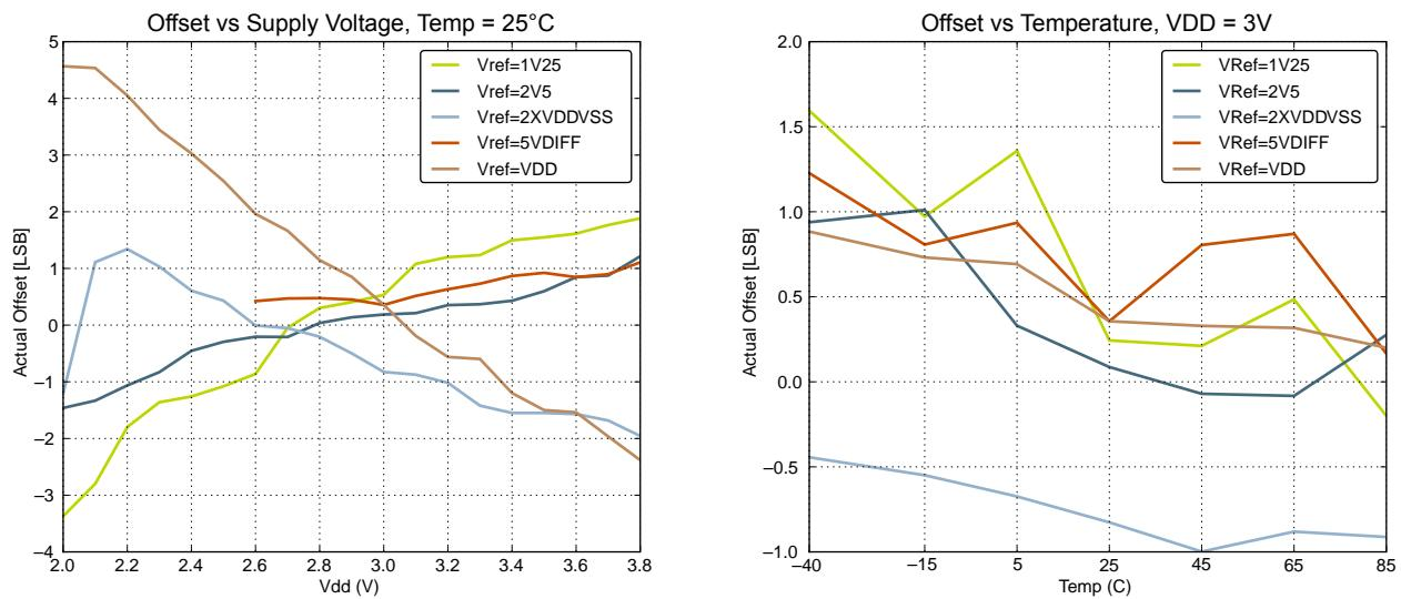
Figure 4.32. ADC Absolute Offset, Common Mode = VDD/2
