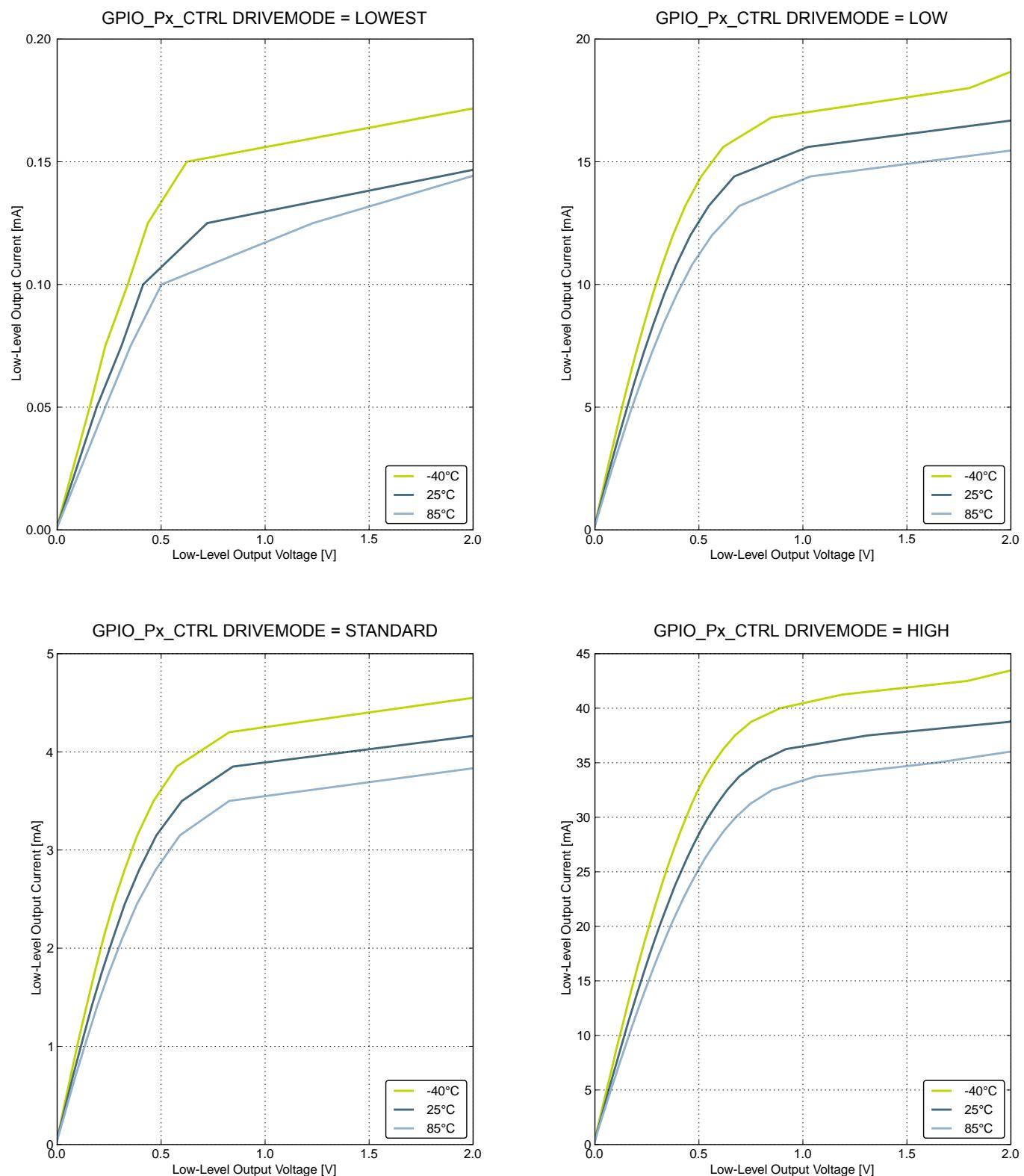
**Figure 4.14. Typical Low-Level Output Current, 2V Supply Voltage**
