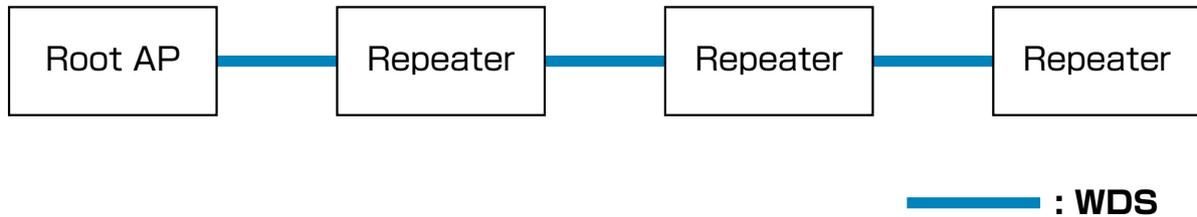
When connecting Access Points, use the first AP as Root AP and the second or later APs as Repeater APs. As shown in below image, connect APs starting from the Root AP.
