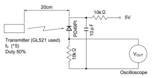
In the above figure, the transmitter should be set so that the output V<sub>OUT (P-P)</sub> can be 40mV. However, the PD49PI to be used here should be of the short-circuit current Isc=2.6  $\mu$  A at Ev =100 lx. (Ev is an illuminance by CIE standard light source A (tungsten lamp).)
