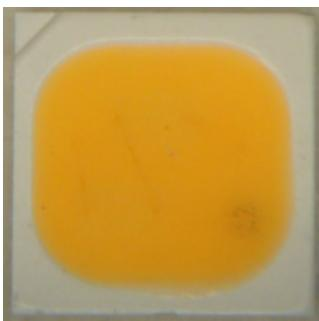
This surface-mount LED comes in standard package dimension. It has a substrate made up of a molded plastic reflector sitting on top of a lead frame. The die is attached within the reflector cavity and the cavity is encapsulated by silicone.
