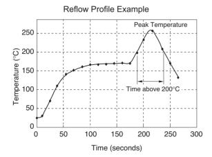
The times of repeated reflow soldering must be two times or less. The Temperature must be measured at top of the cell.
