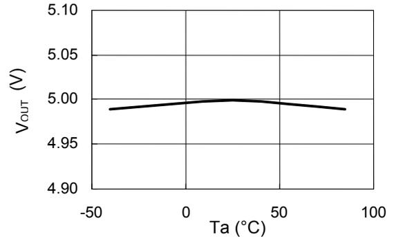
**6. Line Regulation 1 vs. Ambient Temperature**
