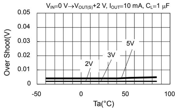
**1.2 At power-on S-817B30A (When using a ceramic capacitor,  $C_L=1 \mu\text{F}$ )**
