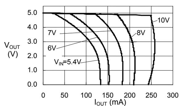
2. Output Voltage vs. Input Voltage
