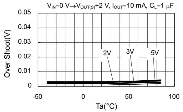
**1.3 At power fluctuation S-817A30A / S-817B30A (When using a ceramic capacitor,  $C_L=1 \mu\text{F}$ )**
