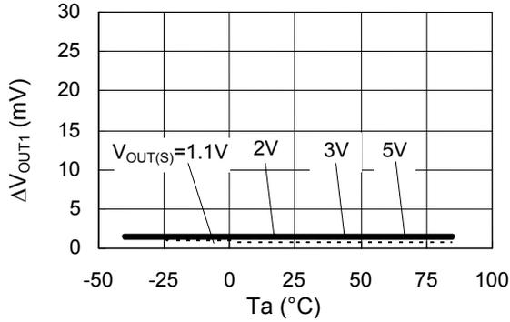
**7. Line Regulation 2 vs. Ambient Temperature**
