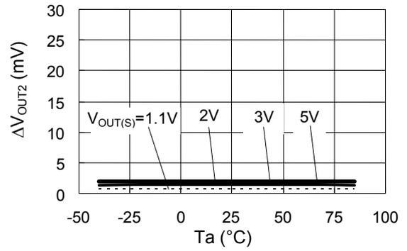
**8. Load Regulation vs. Ambient Temperature**
