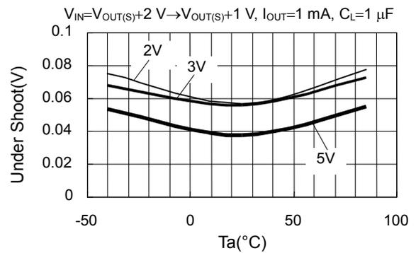
**1.4 At load fluctuation S-817A30A/S-817B30A (When using a ceramic capacitor,  $C_L=1 \mu\text{F}$ )**
