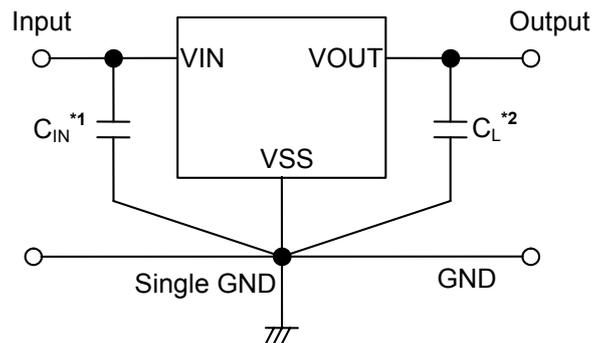
\*1.  $C_{IN}$  is a capacitor for stabilizing the input.
