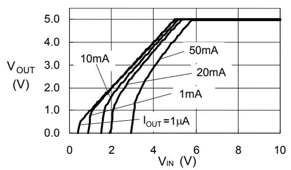
**3. Maximum Output Current vs. Input Voltage**
