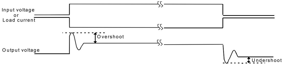
**1.1 At power-on S-817A30A (When using a ceramic capacitor, C<sub>L</sub>=1 μF)**
