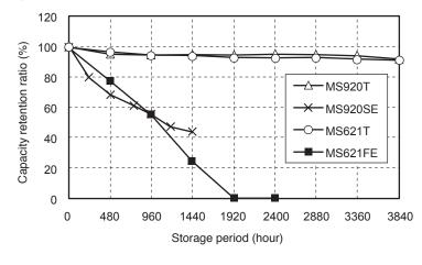
MS-T series' capacity retention ratio after High temperature storage were greatly improved.
