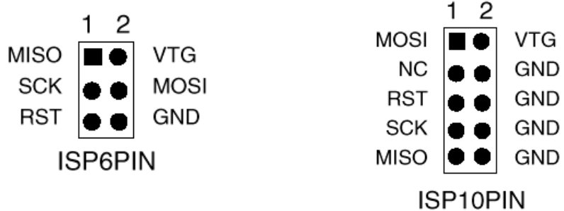
Figure 4-1. Standard ISP connectors on STK500, AVR ISP and STK200/STK300
