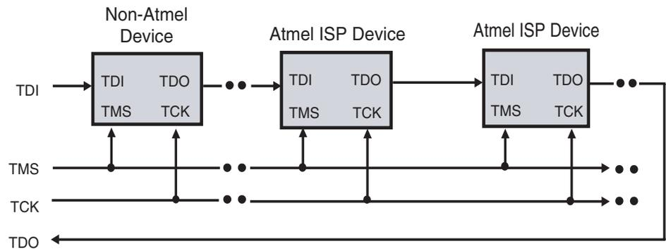
TDI, TMS, TCK and TDO comprise the JTAG interface. The ISP software allows you to create a JTAG daisy chain for multiple devices, including non-Atmel devices, and implement parallel ISP for Atmel devices.
