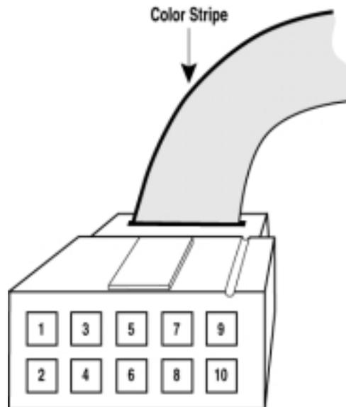
**Note:** Your circuit board must supply  $V_{CC}$  and GND to the Atmel-ISP cable through the 10-pin male header.
