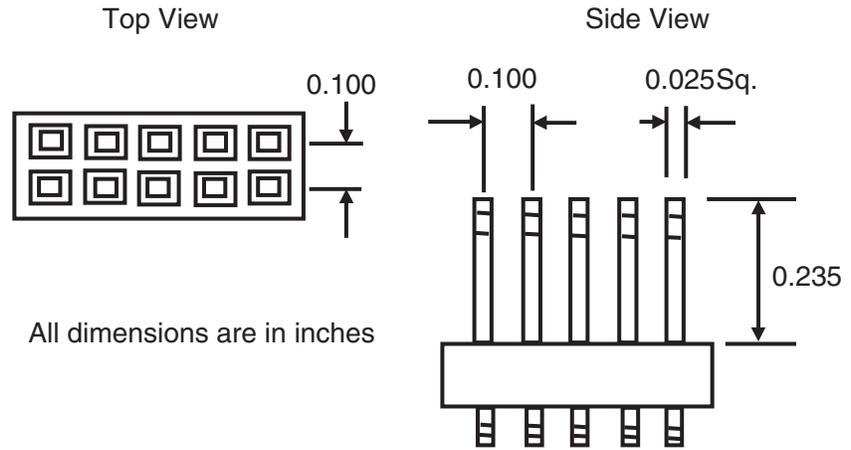
**Figure 4-8.** 10-pin Male Header Pinout
