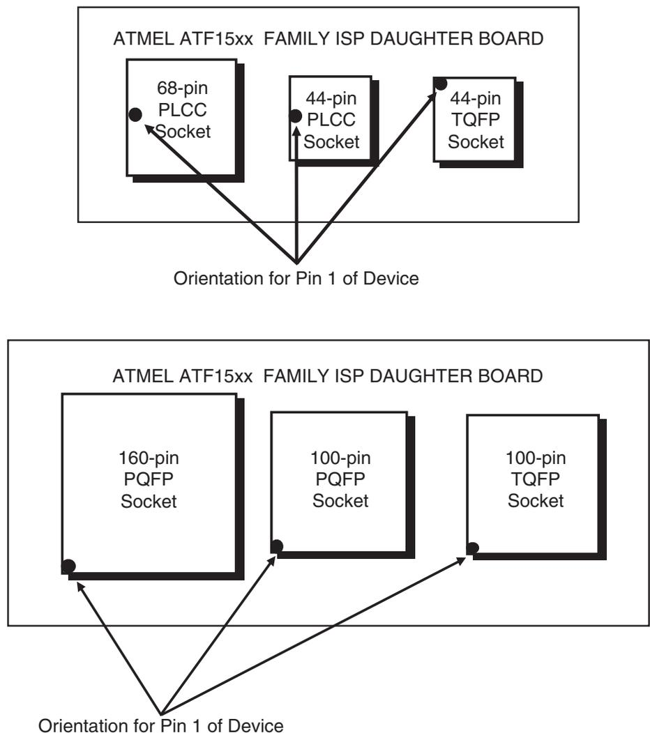
**Figure 4-4.** Correct Orientation of Daughter Board on ISP Board
