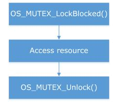
A mutex contains a counter that keeps track of how many times the mutex has been claimed by calling <code>OS\_MUTEX\_Lock()</code> or <code>OS\_MUTEX\_LockBlocked()</code> by a particular task. It is released when that counter reaches zero, which means the <code>OS\_MUTEX\_Unlock()</code> routine must be called exactly the same number of times as <code>OS\_MUTEX\_LockBlocked()</code> or <code>OS\_MUTEX\_Lock()</code>. If it is not, the mutex remains blocked for other tasks.
