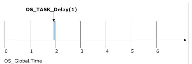
The actual timeout depends on when the API function is called in relation to the next timer interrupt. A timeout of 1 could cause the API function to almost return immediately.
