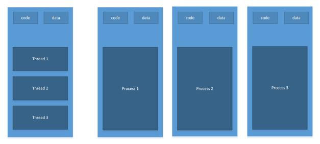
Threads are tasks that share the same memory layout, hence any two threads can access the same memory locations. If virtual memory is used, the same virtual to physical translation and access rights are used.
