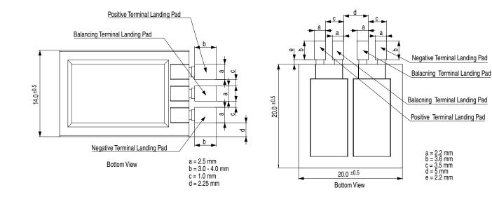
Soldering pads to Case TS20, TS22, TS32, TS35, FS37
