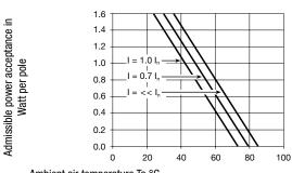
Ambient air temperature Ta  $^{\circ}\text{C}$
