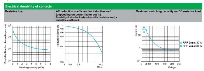
Note: These curves are for reference only and are typical values only. Actual performance is dependant upon the actual load, environment, duty cycle, and other conditions specific to the application.
