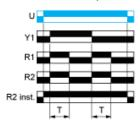
Function C: Off-Delay Relay with Control Signal
