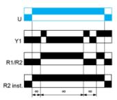
Function Tt: Retriggerable Bistable Relay with Control Signal On
